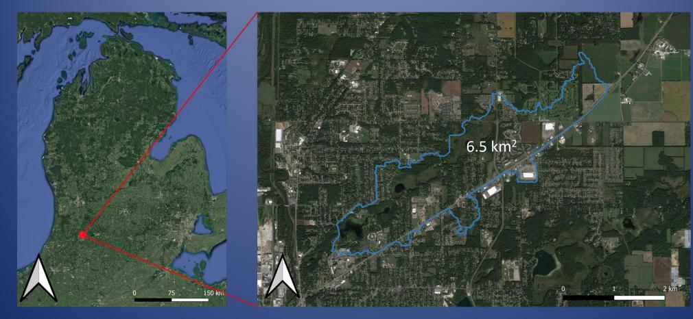
Flow accumulation algorithm in GIS, modified to include engineered stormwater outfalls Provides basis for investigating road salt and nutrients within sub-watershed
